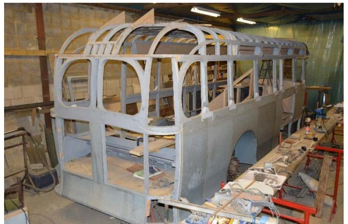
Above and right: From the recovered state (shown on page 1), the body structure was stripped and rebuilt with new ash framing reinforced by steel fitch plates. Much of the original roof, bulkheads and floor was sound and was retained.
