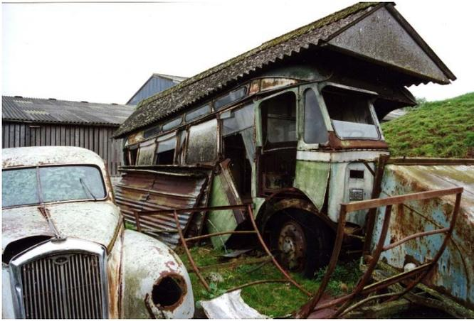
Left and below: 3615 found abandoned on a farm in deepest Somerset. The roof gave some protection from the weather but added significant load causing the body to collapse. Undaunted the restoration team investigates.
