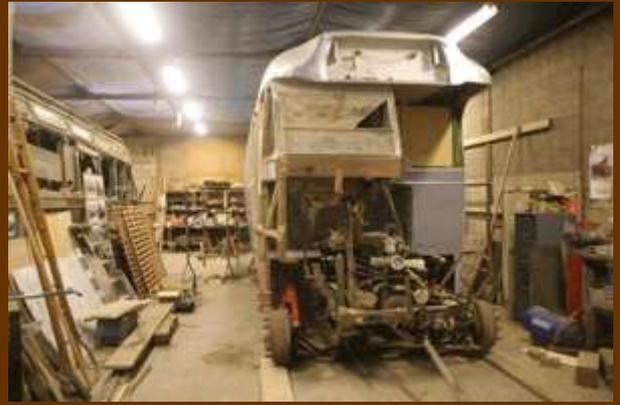
*The chassis has now been lowered to rest on its brake drums on the floor. (Nov 2011)*
