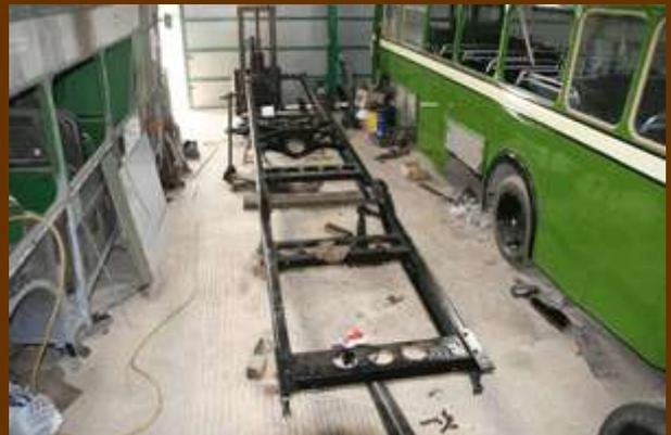
*The straightened, repaired and painted chassis starts to take shape. (May 2012)*
