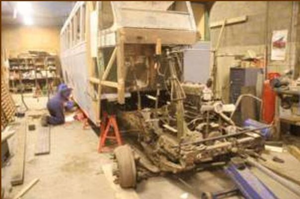
*The chassis begins to emerge by progressively removing and replacing axle stands on either side of the rear axle as the chassis is towed forward. (Nov 2011)*
