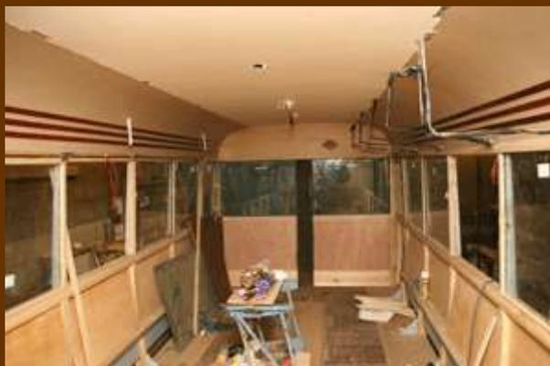
*Head lining and rubbing strips behind the luggage racks are fixed in place and the support brackets for the luggage racks are being fixed in position. (Dec 2012)*
