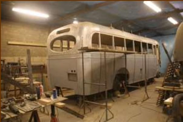
*The body is supported on longitudinal box sections one of which can be seen just to the right of the front offside corner pillar. The box sections are supported on axle stands and, at this stage, the chassis was still in position. (Nov 2011)*
