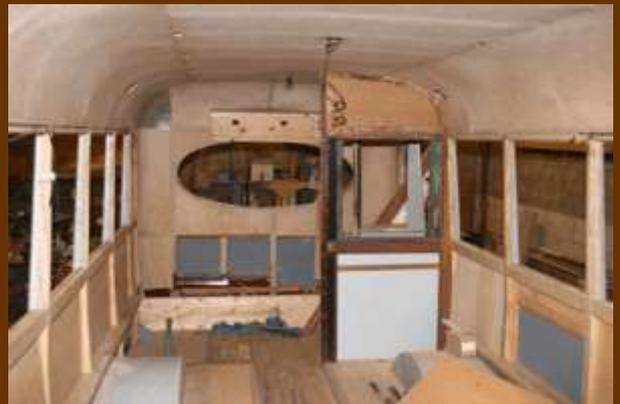
*Interior lining panels in position awaiting trimming. (Jan 2012)*
