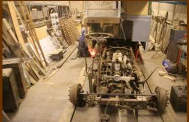
*The chassis is now about half way out with the centre prop-shaft bearing below the saloon front bulkhead. (Nov 2011)*
