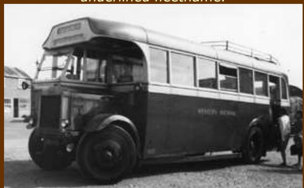
*A later picture of Mumford rebodied PLSC3 No. 2602 with a single half drop window on either side*
