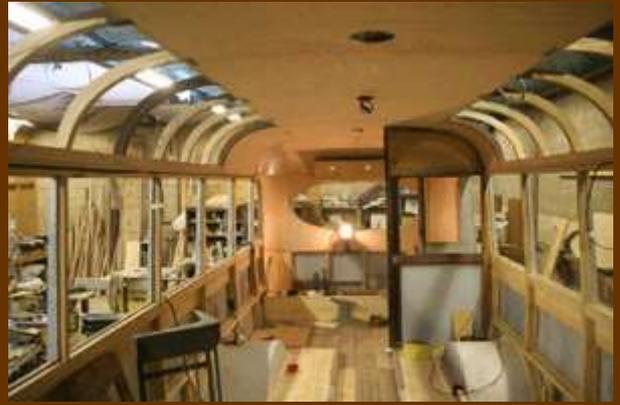
*April 2010. The body wiring was installed before the lining panels. Here, working from the rear the internal ceiling lining panels and external cove panels are being installed.*
