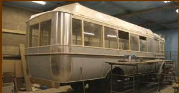
*May 2007. The body with panelling and moulding over the joints complete, windows installed and the large roof rack in place. This demonstrates the use of different materials in the form of construction typical of the late 1920s.*
