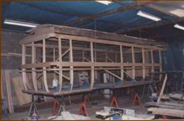
*The body frame taking shape. The original roof can be seen suspended above. Two original pillars were built in on the nearside with other original parts including floor noggins, traps, boarding, front and cab-side bulkheads and many fittings.*
