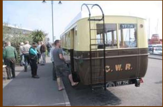
*A rear view showing the wide ladder which unfolds to enable the bottom end to land on the ground and provide a firm footing for the crew to load luggage and goods on the roof mounted rack. Also seen is the 'Hackney Carriage' seating capacity plate, a mandatory requirement before new Licensing and Construction & Use Regulations introduced under the 1930 Road Traffic Act, the single rear lamp and warning triangle reflector. No brake lights were fitted.*
