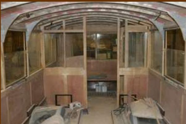
*May 2007. Internal panelling being fitted up before finishing. The internal finishing was an 'ivory' painted roof with structure and panelling below the cant rail stained and varnished and floor under the seats covered in brown lino and aisle and luggage compartment floor painted brown.*
