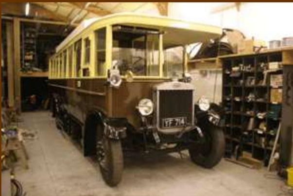
*December 2010 with completion in sight. Lining out and sign-writing complete, electrical installation almost complete, advance and retard and hand throttle linkages in final stages to enable completion of the cab floor and installation of drivers seat. Outstanding items: bell and chord, passenger door latch and bolting system, spare wheel carrier, mirrors, traffic notice board, destination board.*
