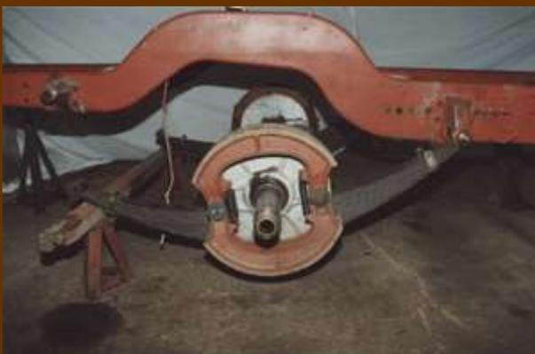
*Rear axle being installed on new road springs with new shackle pins and bushes. The original brake shoes have been relined and new brake cams and pull-off springs fitted.*
